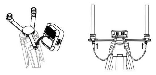
3. Install the antenna on the tripod, and connect the antenna feeder to the base station antenna port.
