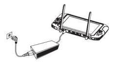
To charge the ground station, connect the round head line on the charger with the ground station.
