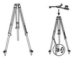
2. Install the base station main body on the tripod and screw up the locking nut on the main body, to ensure that the base station is horizontal and firm.
