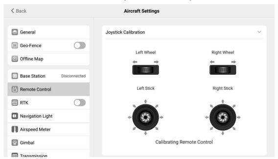
3. Follow the direction of the arrow on the screen, turn the roller clockwise and hold for 1 second until you hear a beep, then turn it counterclockwise until you hear a beep. Next push and hold the rockers in eight directions one by one until you hear a beep every time. When the ground station no longer emits the rapid and intermittent beep or the screen shows "Calibration completed", it means that the calibration has been completed.
