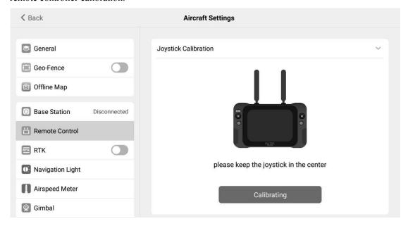
2. Select "Calibrate". The left and right rollers and left Right rocker legend will appear on the screen, and the remote control will emit a rapid and intermittent beep.
