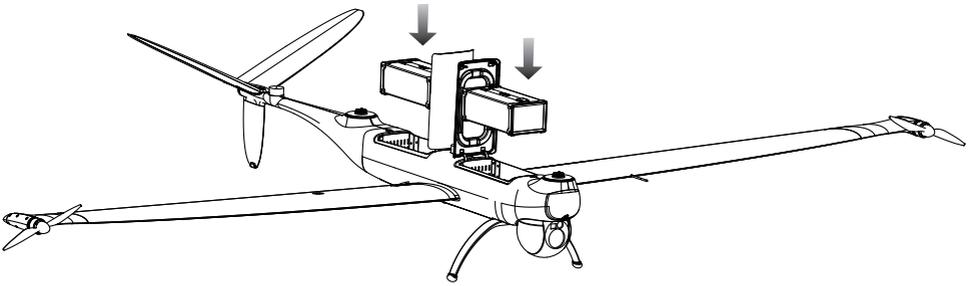
Align the battery to the battery interface on the fuselage and install it.
