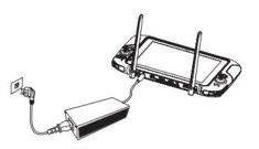
To charge the ground station, connect the round head line on the charger with the ground station.
