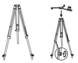
2. Install the base station main body on the tripod and screw up the locking nut on the main body, to ensure that the base station is horizontal and firm.
