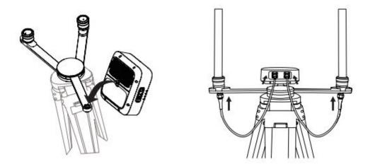
3. Install the antenna on the tripod, and connect the antenna feeder to the base station antenna port.
